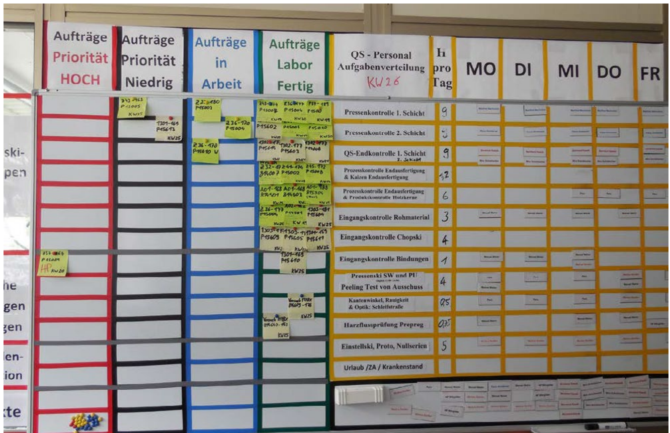
This Kanban board keeps track of the quality tests for various pairs of skis. Inspired by IT’s Kanban board, it is one of the latest improvements on the manufacturing floor.
